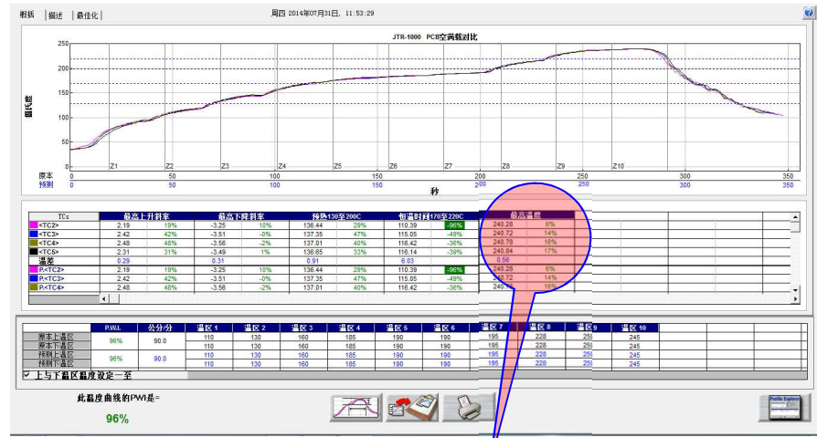
Fully loaded PCB board temperature curve
